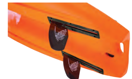
Retractable twin fins for directional stability and ease of storage.
